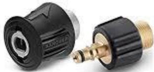
The first adapter is a female K2 x Female M22/14mm. Once you have this adapter, you can use a Male M22/14mm x Female 3/8" Quick Connect fitting.
